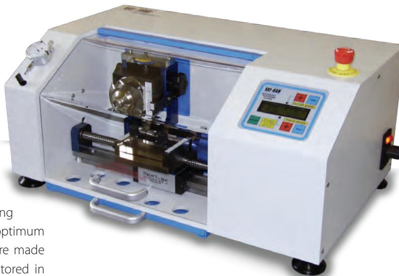
and provides an electrical interlock so the machine does not operate when the guard is open.
