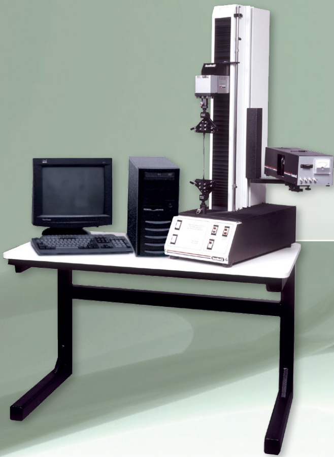
United SSTM "SMART" Table Model, Single Column shown with optional United Lazer Extensometer
